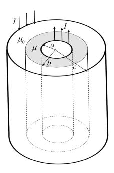
(a) Choose an appropriate coordinate system and, using Ampere's law, show that the magnetic field everywhere in the region  $a < \rho < b$  is given by
